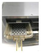
Remove tray seals by lifting up on the tab and then sliding the tray seal out of the cabinet.
